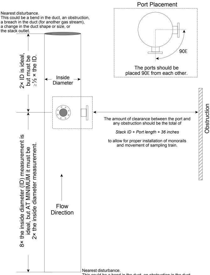
This could be a bend in the duct, an obstruction in the duct, a breach in the duct (for another gas stream), or a change in the duct shape or size.
